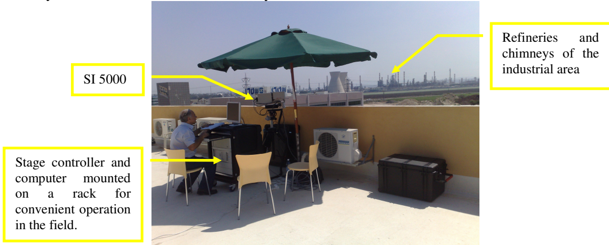
Figure 2: The operational SI 5000 shown mounted on a tripod (under the umbrella), and measuring the gas emissions from the Haifa refineries and fertilizer producers' smoke stacks. The author of this paper is at the system controls.
